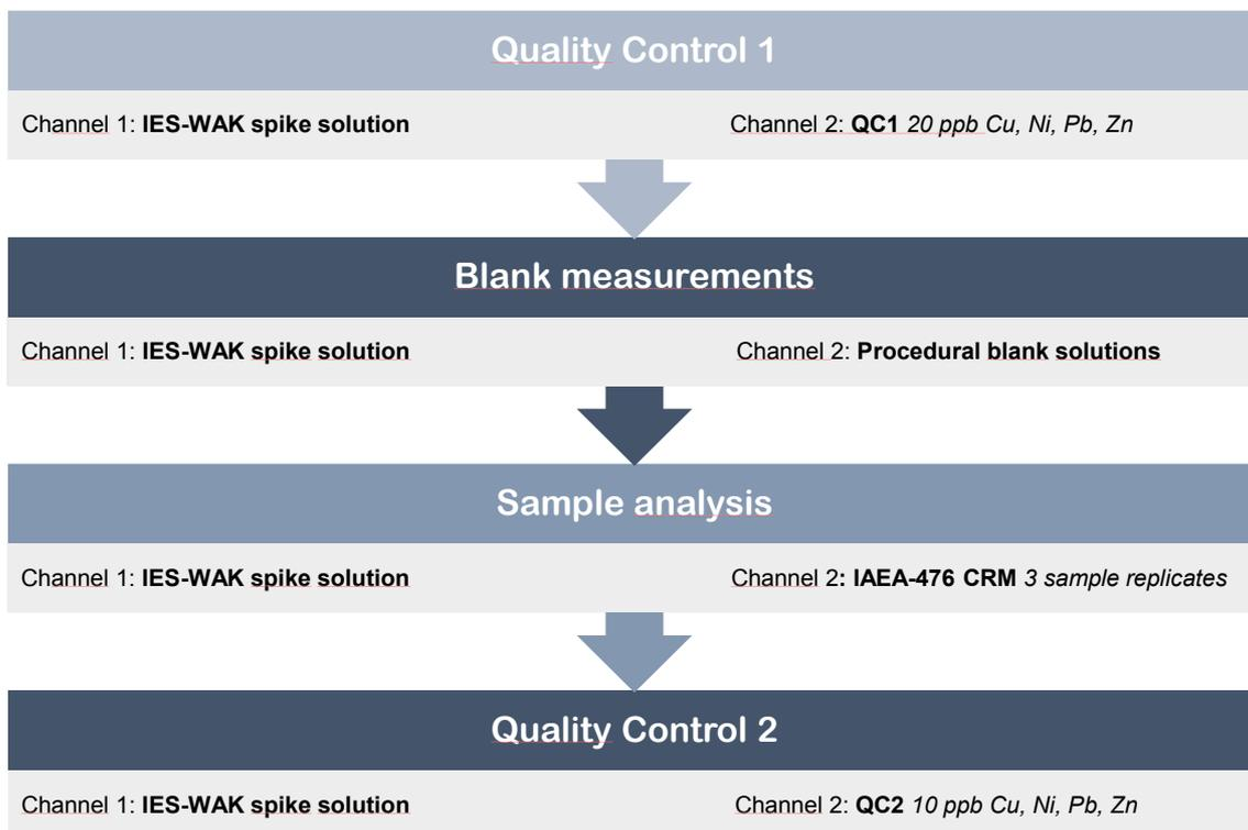
**Figure 3.** Analytical procedure for the on-line isotope dilution analysis using the MultiNeb<sup>®</sup> nebulizer with two independent liquid inlets (Channel 1 and 2).
