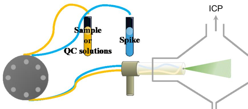
**Figure 2.** Scheme of the on-line isotope dilution system using the MultiNeb<sup>®</sup>.
