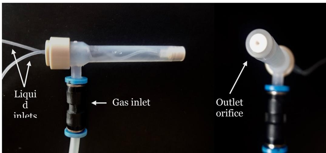
**Figure 1.** Side view (left) and front view (right) of the MultiNeb<sup>®</sup> multiple nebulizer prototype.
